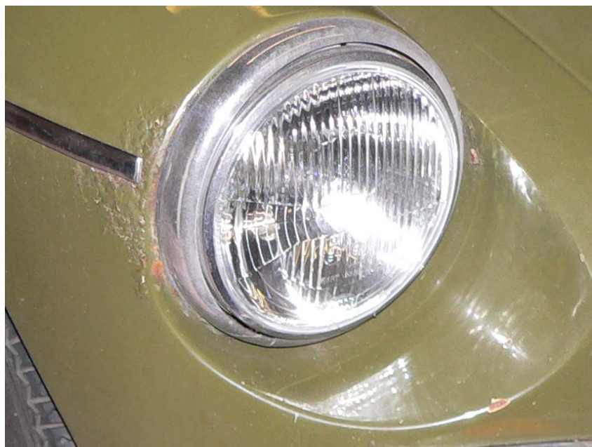
Some rust showing around the offside headlamp
