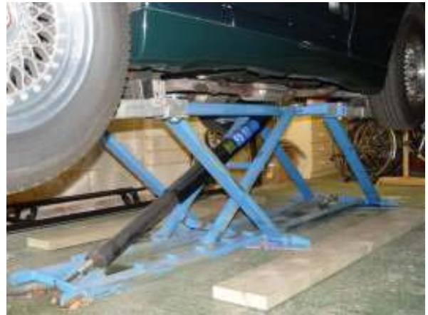
The Autec ramp lifts the car well clear of the ground. (Photo: Gavin Bailey)
