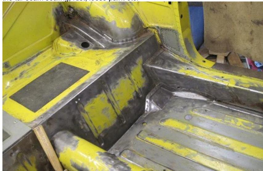
The parts I could not get to with the knotted wire brush on the angle grinder I scraped the tar off with a scraper and cleaned the rest of the tar off with thinners.
