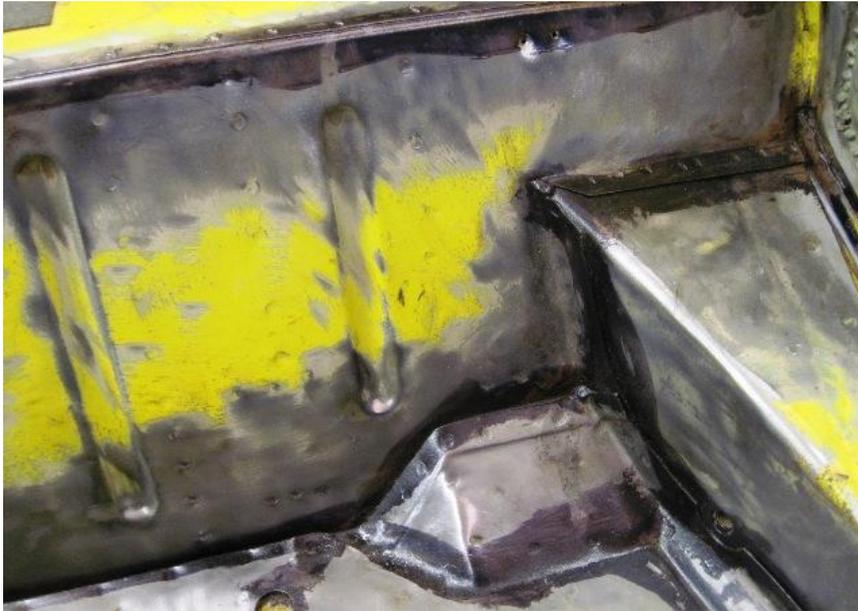
Overnight the Kurust worked a treat in the cleaned out seams. It is now ready for a coat of etching primer over all the bare metal bits.
