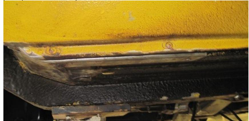
These screws at the bottom of the wings are usually an absolute pain to remove. I have sprayed them well with penetrating oil before I even attempt to undo them.
