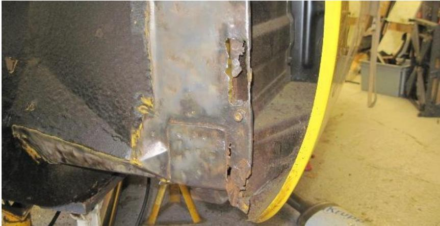
While I had the wire brush on the angle grinder I looked for some other parts that needed repair. This front LH panel where the splash guard goes showed some rust holes, even more when all the underseal and paint were removed. To make the welding job easier the front wing needs to be removed.
