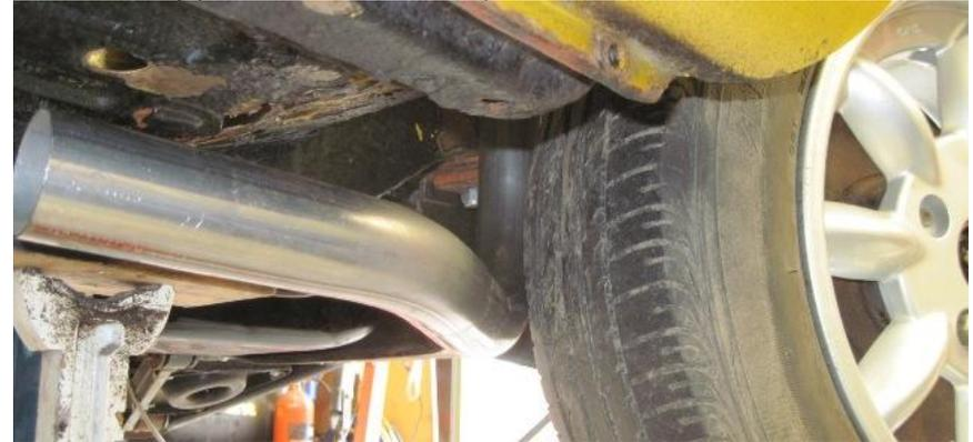
Refitted the down pipe from the other side and no problems, but of course the exhaust run is back on the inner side of the chassis rail.
