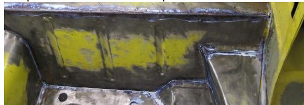
The seams were coated liberally with Kurust, so hopefully the Kurust would soak into the seams. I will leave this overnight to work and then coat with etching primer.
