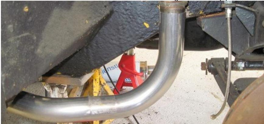
It fits nicely in the position but will the 15" Minilite wheel with the 15 x 195/65 tyre foul the exhaust on lock. Before I tried the wheel and tyre I needed to be able to turn the steering wheel. I had only put a temporary nut and bolt in the steering UJ and it was fouling on the exhaust manifold because it was too long. I shortened the bolt to the correct length.
