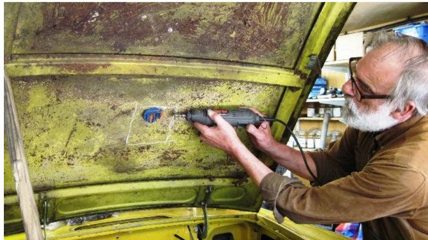
Attacking the hole in the bonnet with the Dremel cutting disc. John then said "Don't ponce around with that tool, it will take ages. Use the angle grinder with the 1mm cutting disc". He was right again – the angle grinder soon cut through the bonnet.
