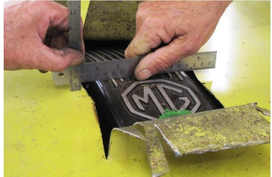
At last they managed to measure it accurately, 10mm above the top of the bonnet. We all agreed that 15mm clearance would be sufficient. I suggested that I could panel beat the bonnet up by 15mm over a large enough area without it looking different to a standard bonnet. Shouted down again I agreed to machine 15mm off the manifold or trumpet stack or both. Mind you I may have a look again at the engine mountings and see if they will recess into the chassis rails – but don't tell them!
