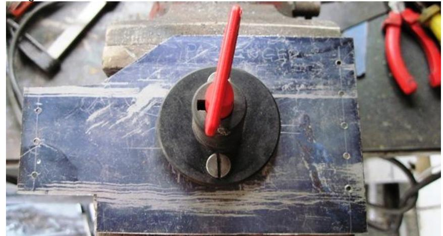
The battery cut-off switch finally screwed to the new panel. Ready to blast, clean and paint with self etching primer before being fitted into the body shell, I am going to rivet this plate in place rather than weld it just in case it fouls with anything.
