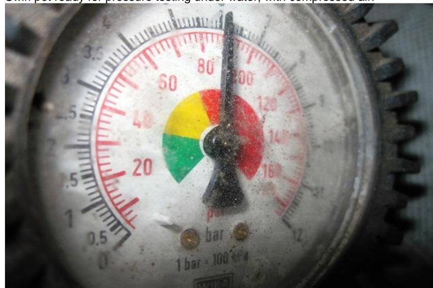
It was difficult taking a photo with one hand and holding the tyre pressure gauge with the other. I did take it up to 100 psi but as you can see the gauge in the picture is just under 90 psi. Good enough to show any leaks. After looking for a tyre valve for about 5 minutes I gave up and used a tyre valve extension. This is a part with which you can extend tyre valves if they are too short to get the tyre pump onto. I fitted this into the rubber hose and firmly connected it again with a
