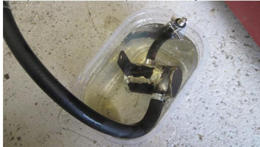
Swirl pot ready for pressure testing under water, with compressed air.
