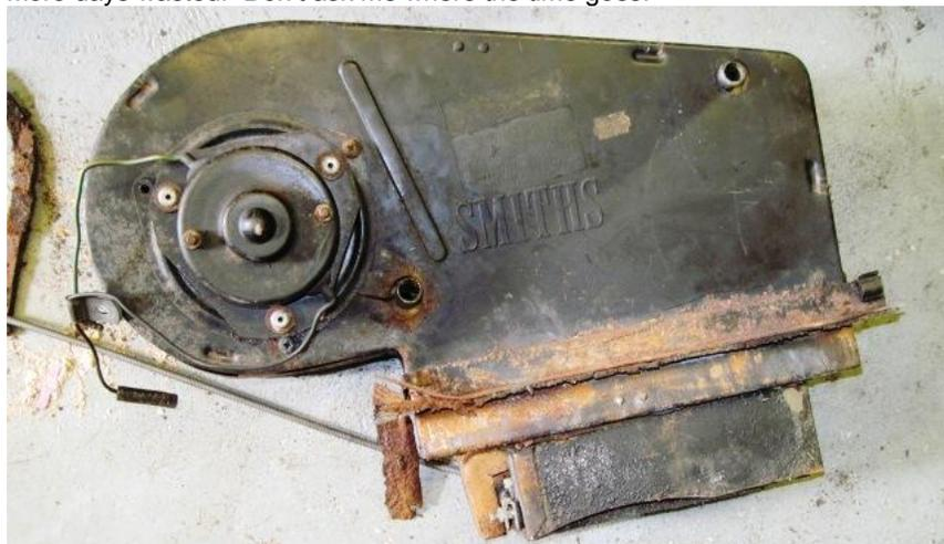
As I don't seem to be able to get on with the yellow MGB at the present time, I thought I would finish off this page with some details of the teal blue MGBGT V8 that I sold back to Dugald. The first photo is of the heater assembly as it came out of the car. You can see that casing was split at the front where one of the heater pipes comes out. I decided to buy another heater off eBay and use the best parts to make one good heater
