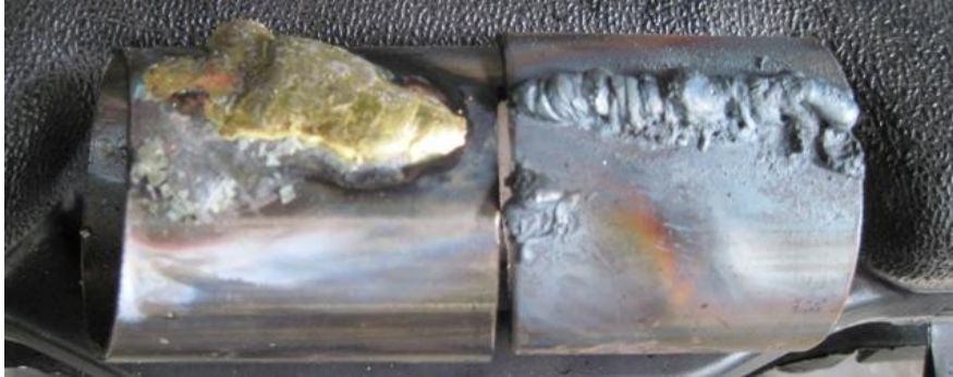
How not to gas weld or nickel bronze weld!
