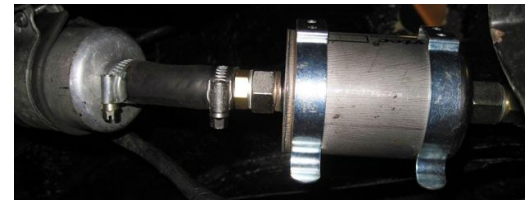
The pump and swirl pot in position and ready for making a bracket for the pot. It looks as if it will line up nicely with the fuel line to the engine.
