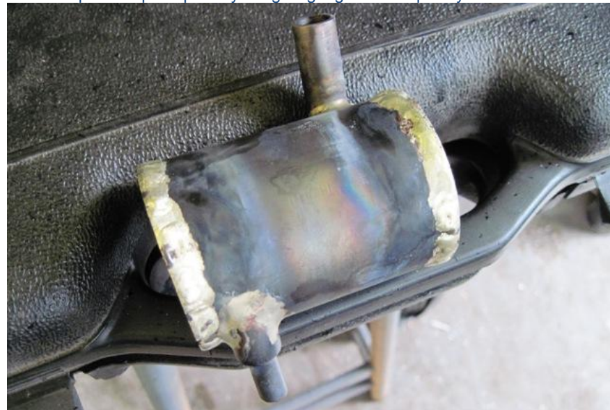
The swirl pot clamped up ready for 'gluing together'. Hopefully with no leaks.
