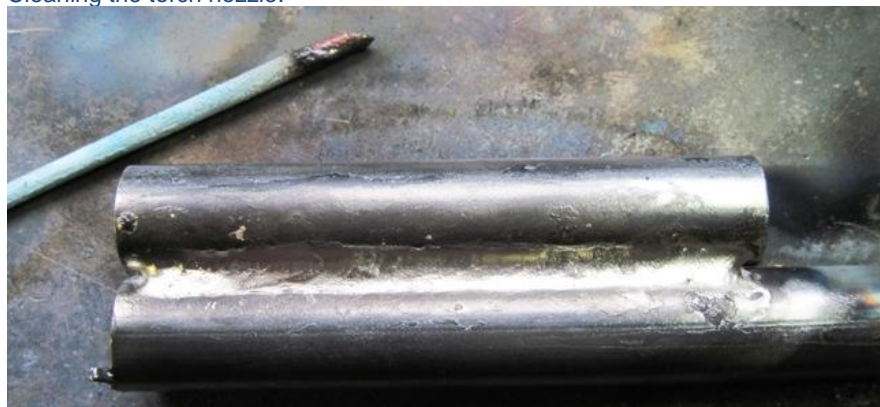
Weld with the blue fluxed rod.
