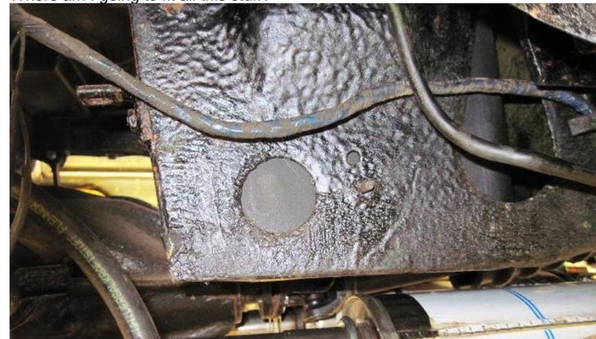
The side of the battery box looks suitable. It also has some threaded studs sticking out that may help with the mounting of some of the fuel system parts.
