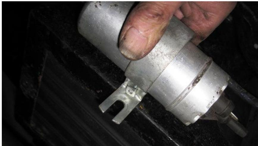
The fuel pump did not have a mounting. Instead of making a bracket I thought a clamp for an ignition coil would do. I found one in one of my boxes of car stuff. It seemed perfect as it is slightly oversize and so I will be able to fit a ring of rubber between the coli clip and the fuel pump. I must remember to test the pump and find out the fuel delivery to check that is suitable for the injection system and a 3.9 litre engine.
