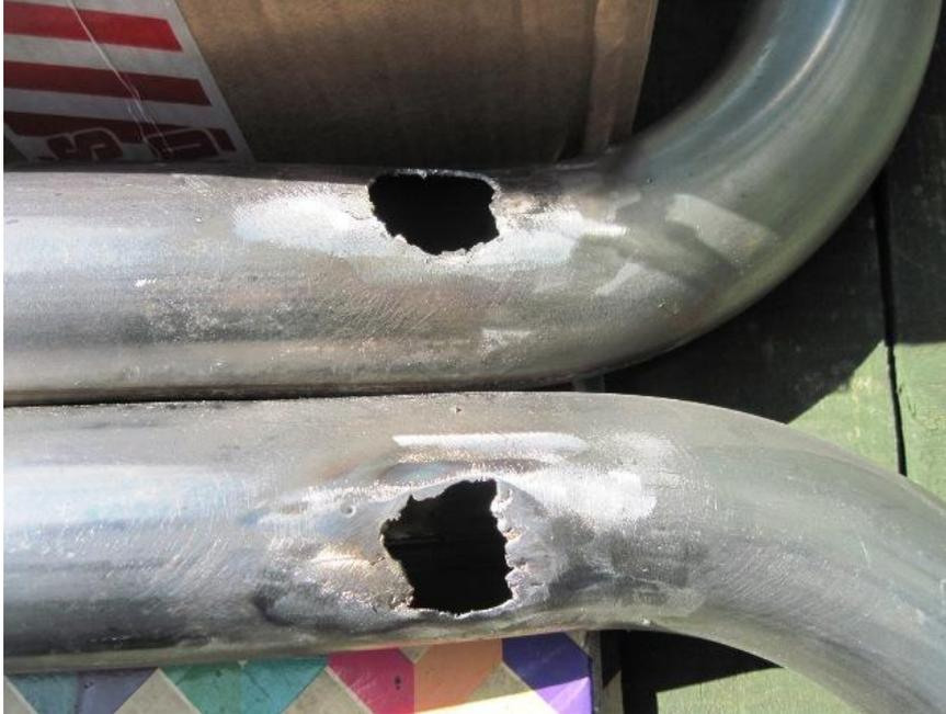
I wrote down a few ideas in my book of how to get over the problem. Decided that as I had a mild steel bend that had a section on it that would fit over the 2" diameter down pipe I would make two new collars for the oxygen sensors out of mild steel and weld them to plates made out of the larger section of the mild steel bend.
