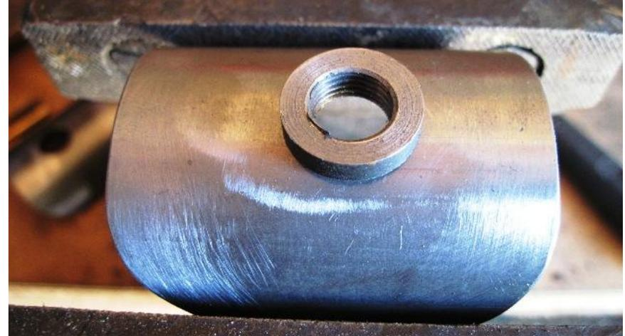
The patch was now ready for welding the collar into it, the patch could then be welded over what is now a much larger hole than they should have been, in the exhaust down pipe. Never mind - these problems come to try out my patience and get me thinking. It least it stirs up the old grey matter in the brain!
