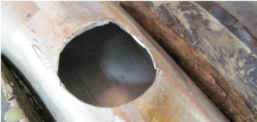
I cleaned out the jagged holes as best I could. Made the new collars in the lathe and threaded them as before. These would be welded to the sections of 2" plus
