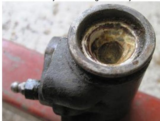
That's what you call a seized wheel cylinder. With an MGB you would just buy a new one. A bit of a problem finding a new one for a 1934 car! You just have to unseize it and hone out the bore. The seals were fine to reuse.
