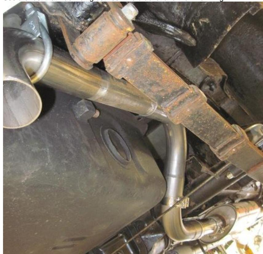
I finished making the pattern for the RH tail pipe from the silencer, although I would like to make a third mounting just behind the silencer. Thought the pattern would do for the LH side as well. I will have to think about this.
