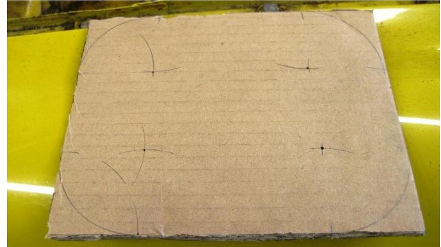
I then held the cardboard up to the hole and measured and marked how much room I needed around the hole for fixings. I then stuck some thinner cardboard on the back with masking tape. Marked out the position of the fuse and relay boxes.
