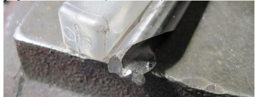
The working end of the spot weld drill.
