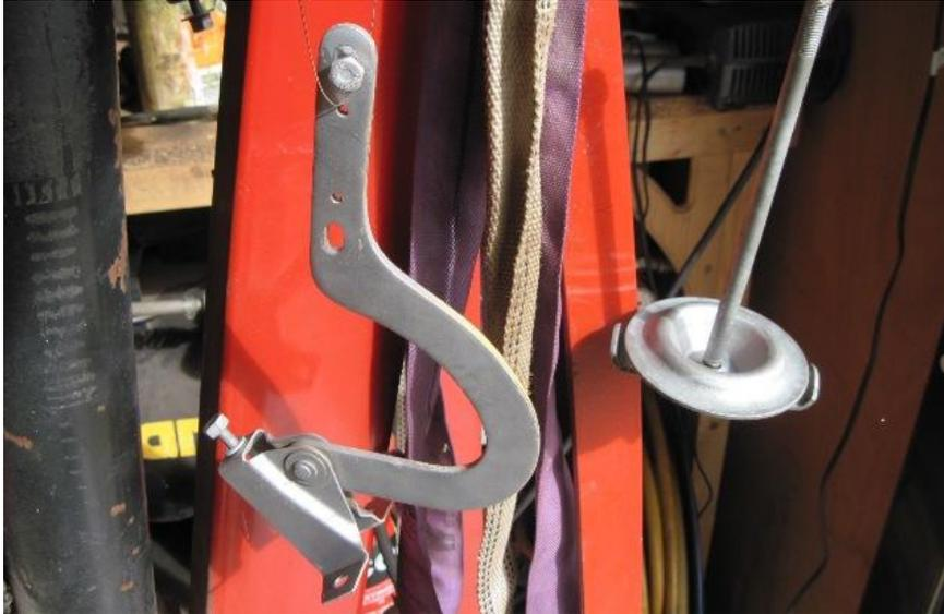
Hinge and spare wheel clamp, blasted and ready for etching primer.
