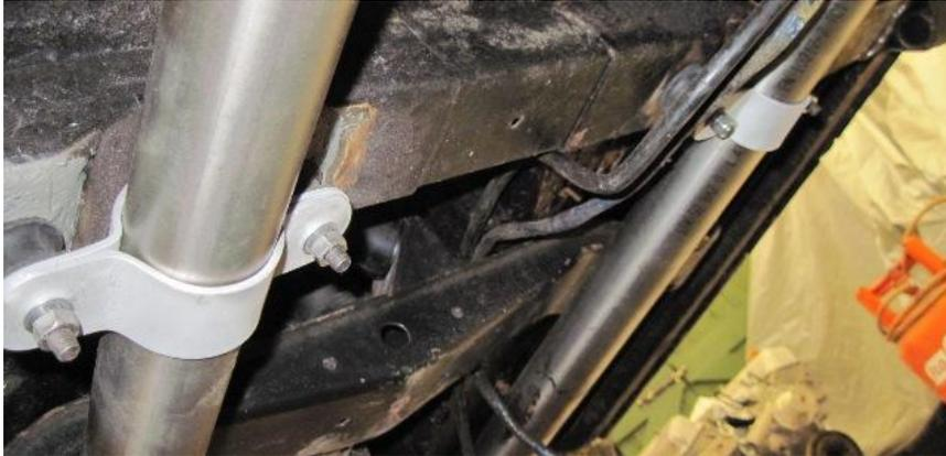
The two forward exhaust mounting brackets in 1/8" aluminium plate, finished at last. Yes, I will cut off the extra thread sticking out of the cotton reels.
