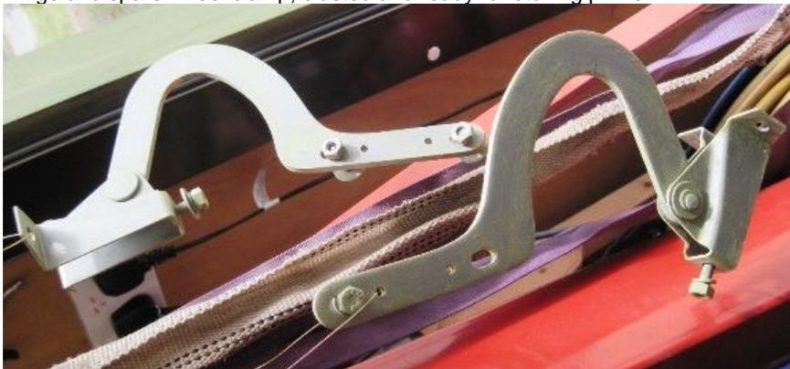
Hinges, freed off, blasted and painted with etch primer painted on with a brush. You don't need a lot of paint, only a light covering, enough to stop the parts rusting again before they have the primer and top coat. Sorry about the photo being sideways. I did it this way so I could fit some writing in. Some people might say they prefer me not to write but just have photos.
