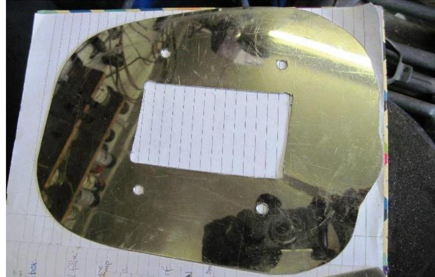
This is the back of the plate before deburring the holes and the centre hole.
