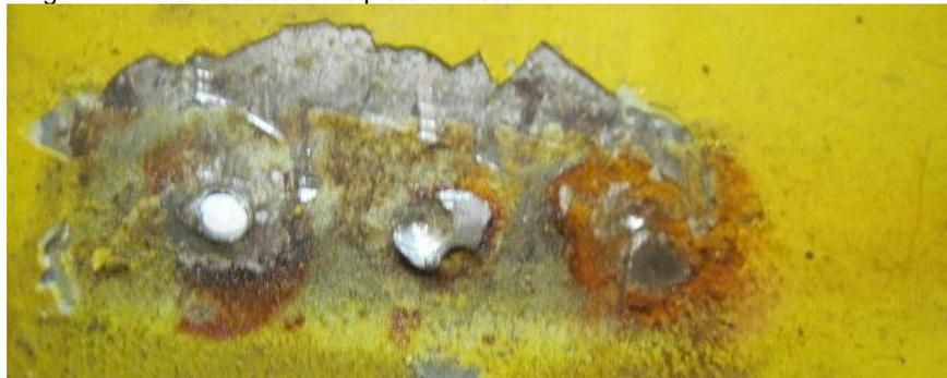
See the rust that was hiding between the bracket and the inner wing.
