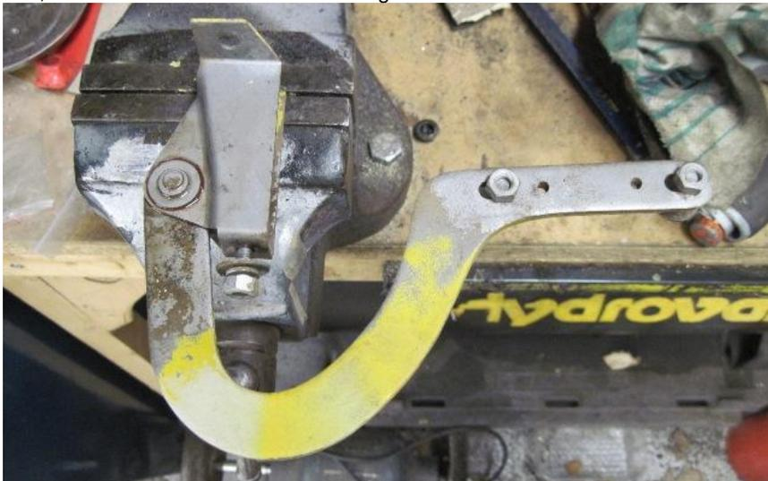
I blasted the area around the **hinge pin** and then soaked the area in penetrating oil. Left the oil for about an hour and then kept moving the hinge to loosen it off. I will wipe off the excess penetrating oil and blast the rest of the hinge.
