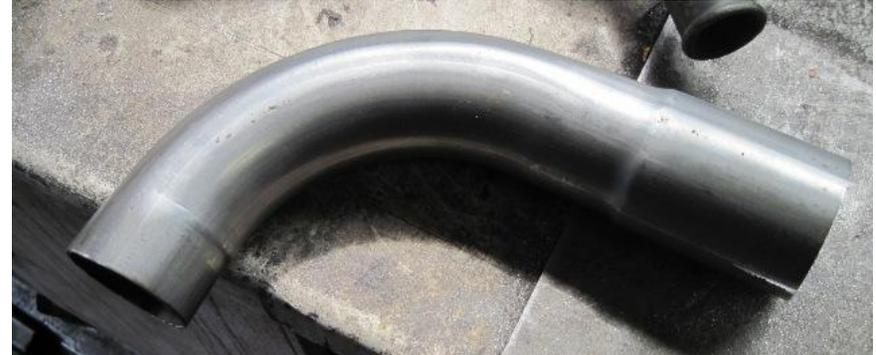
The 90 degree bend cut to size with the 1mm cutting disc.
