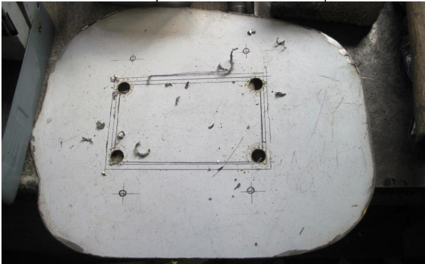
After marking the position of the hole in the centre and the mounting holes for the boxes, I drilled out the corner holes with a 10mm drill as I did not want sharp corners of the square hole. The stainless plate was then cut out using the angle grinder and cutting disc. The more you do of this sort of job the easier it gets.
