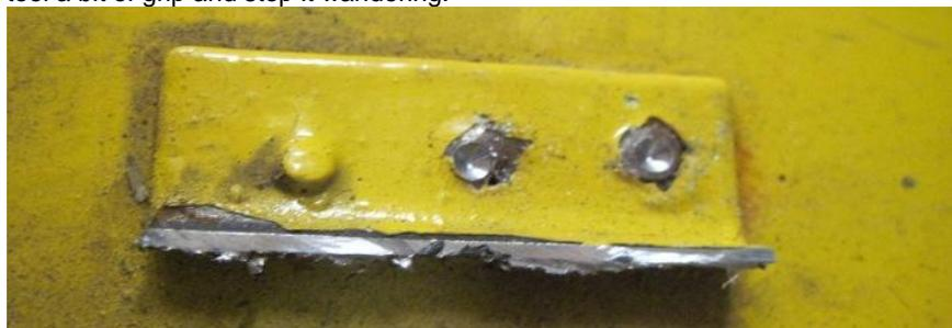
Drilled through the top surface with the spot weld drill. Don't go too deep or you will have holes to weld up. The peg sticking up is a location marker for when the bracket was originally fitted to the inner wing to make sure it was fitted in the correct place.
