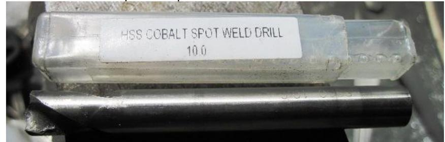
This is a 10mm Cobalt spot weld drill. Buy good quality spot weld drills if you are going to have to drill out a lot of spot welds as cheap drills last know time at all.
