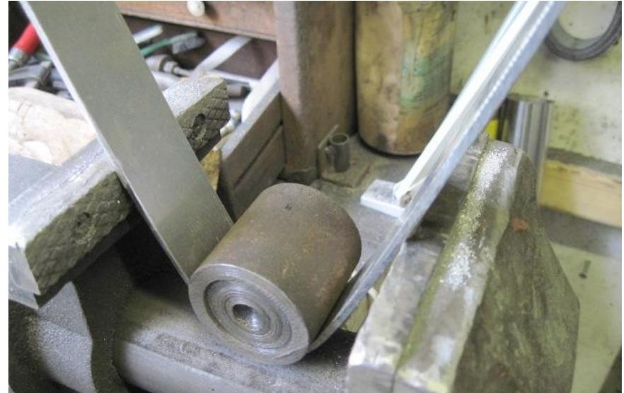
Bending the aluminium strip around a 2" diameter bit of bar in the vice. I tried using soft vice jaw covers, but they kept slipping out.
