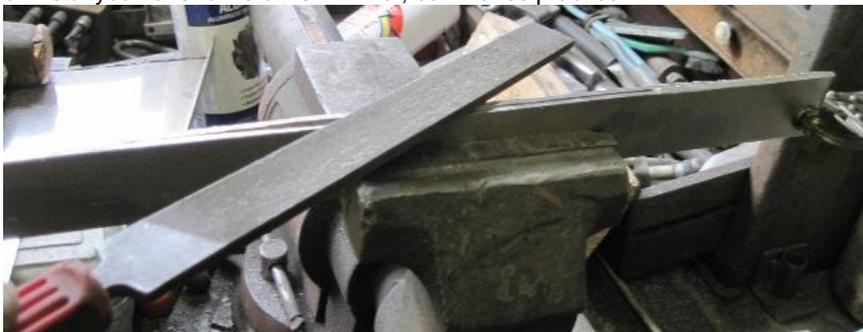
Filing the rough edges off the disc cut aluminium plate. When filing aluminium you need to use a file card to remove the bits of aluminium out of the file grooves on a fairly regular basis, otherwise the file clogs up.
