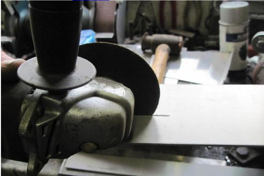
Cutting the aluminium plate into strips for the exhaust mounting brackets. With the disc cutter you can get very close to the scribed line on the plate and the amount of metal you have to file off is minimal, but it takes practice.
