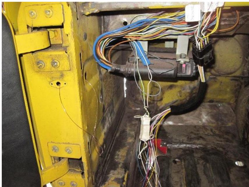
The wires from the engine loom that go to the ECU and the other wires that go to the dashboard etc. will all be loomed up after we know the engine runs and everything is working properly.
