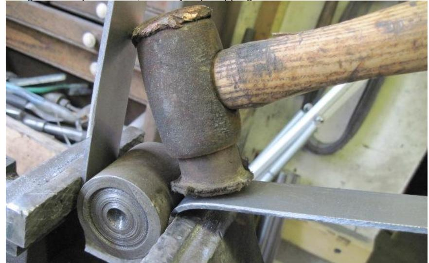
Bending the exhaust mounting brackets into shape with the hide side of a copper/hide mallet. The other side of this bracket is harder to bend in the vice. I apologise if this report is a bit boring for those that know about metalwork. There are many who think restoration and building cars is witchcraft, so I am trying in my reports to cater for everyone. Comments, abuse, questions etc. to [mikemacartney@btconnect.com](mailto:mikemacartney@btconnect.com)
