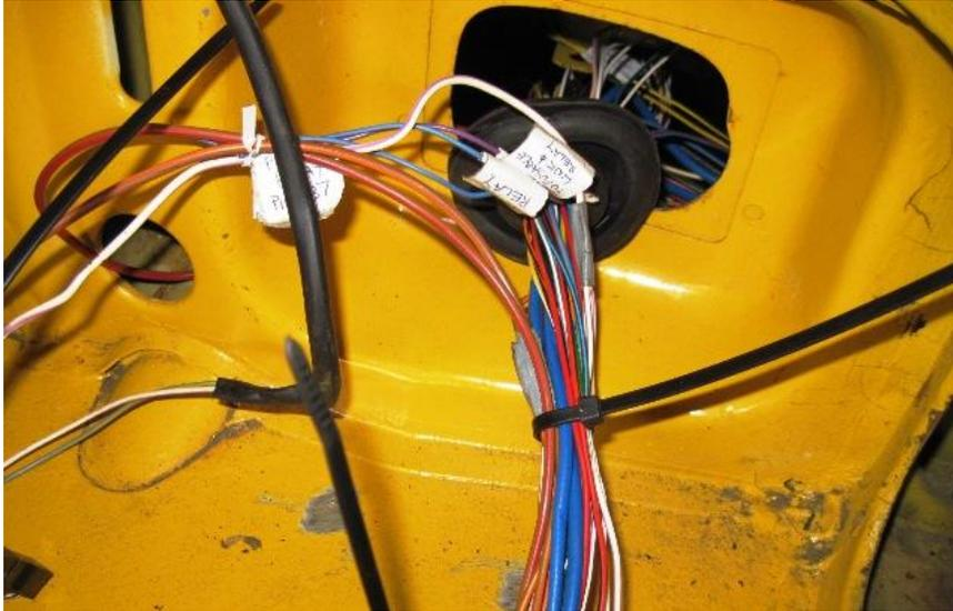
Wires routed as to whether or not they go inside the passengers compartment or into the engine compartment. He likes to use reusable cable ties to temporarily keep the wires that are going to the same area together.
