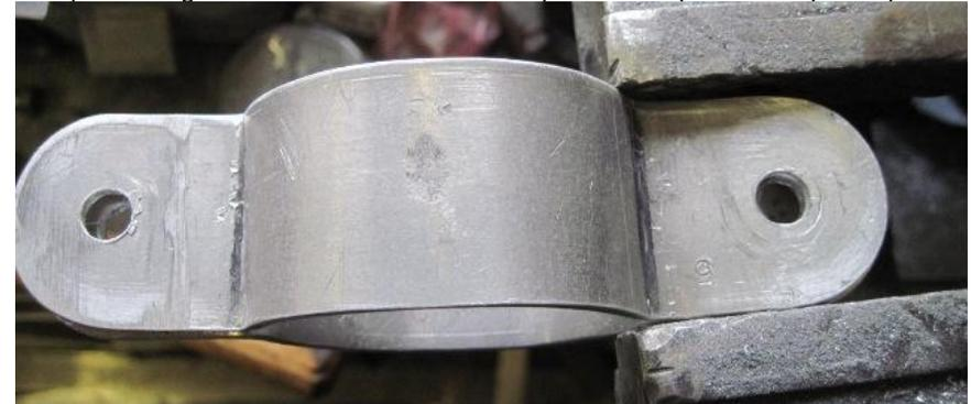
The next job was to file and clean the clamp to a reasonable finish and check that it clamped still clamped the 2" stainless steel exhaust pipe.
