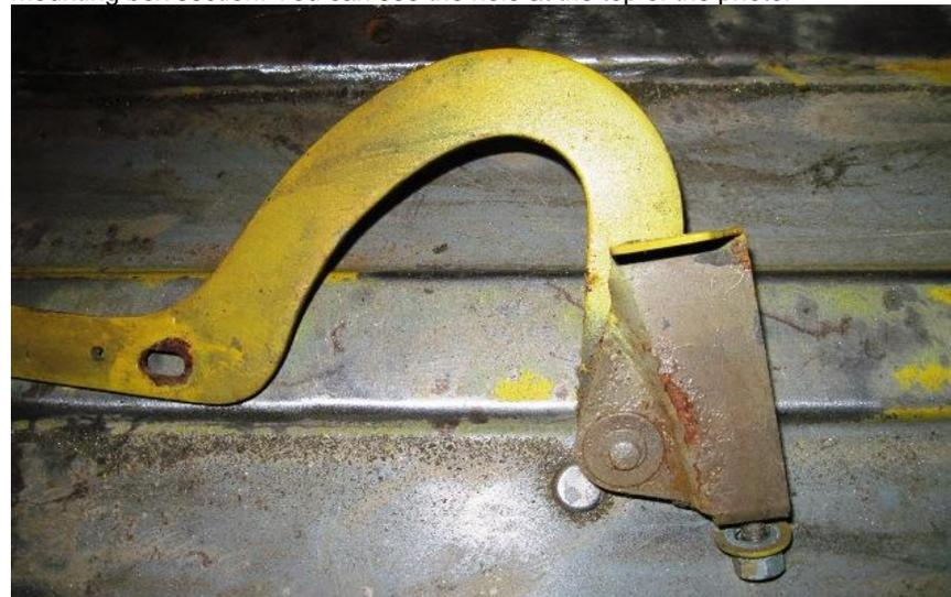
You can see that the hinge was never painted with top coat, only some sort of transit primer. I will try blasting it in the cabinet to remove the rust and if that does not free off the hinge I may have to drill out the hinge pin and clean up the parts and rivet the lot together again. I will paint and oil the hinges before I refit them. Hopefully then they will last another forty odd years.
