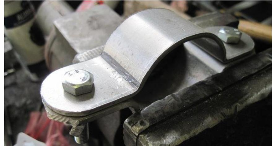
Finished of the top clamp, and drilled the 5/16" clearance holes. Put the top clamp on the bottom clamp. Drill a hole at one end of the bottom clamp and bolted the two clamps together. I was then able to hold the other end of the two parts of the clamp together with mole grips and drill the second hole. Install the second bolt to clamp them together and cut the bottom clamp to the shape of the top clamp.
