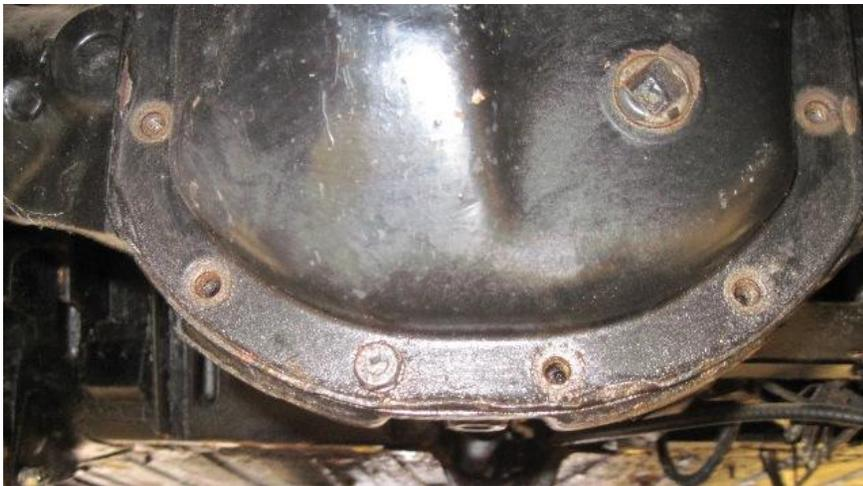
With the rear axle hanging down I could get on with setting up the exhaust for mounting. Why are there only 2-bolts holding the differential back plate on? I better investigate this when the exhaust position and mounting is completed. Supposedly, the diff has been fitted with a Quaife limiting slip diff. I dug out the new stainless steel exhaust silencers and stainless steel exhaust piping that came with the MG.
