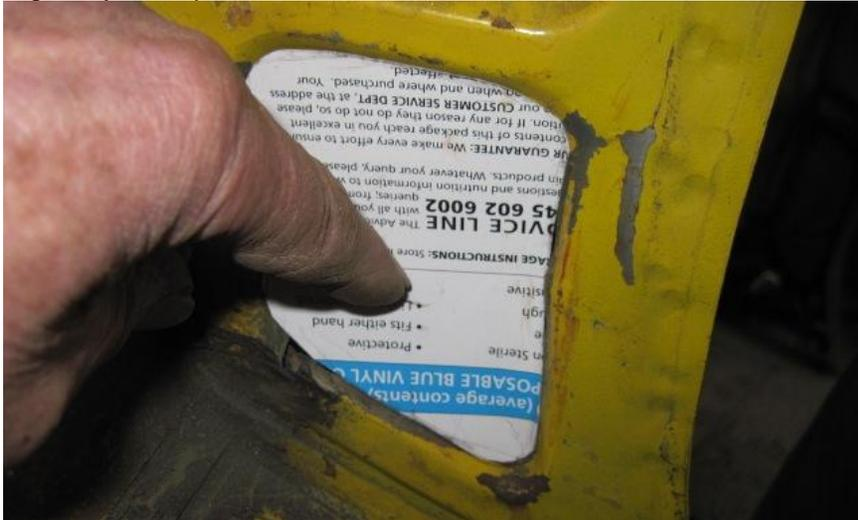
In the past somebody had hacked out this part of the inner panel behind the door shut. Although it is hidden I know it's there, decided I would fill the hole back in with a plate to help with the structural strength.
