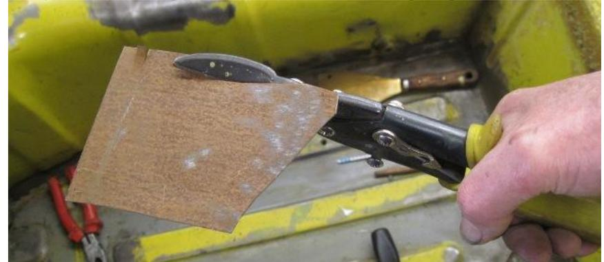
Cut out the plate with the snips. There are three snips in a set. One pair for cutting in a straight line, one for left hand curves, one for right hand curves. I did blast this plate before I welded it in place.
