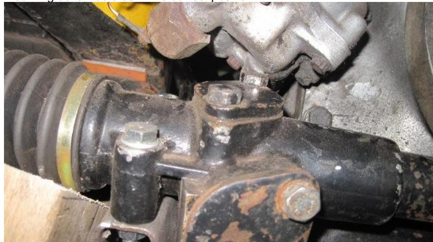
The rear bolt on top of the steering rack is very close to the oil pump base. Not a problem as I will remove it when the rack is out of the car, countersink the hole in the top plate and fit a socket head countersunk 5/16" UNF bolt.
