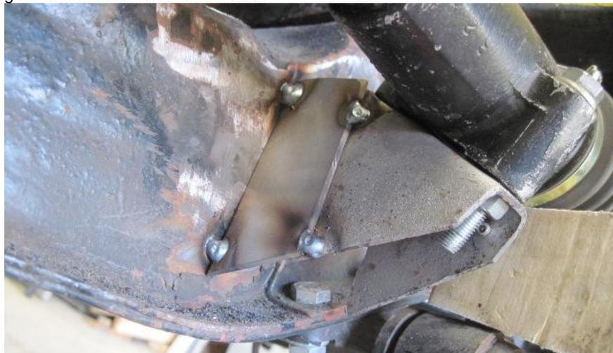
The plate for the rack mounting tacked in position.
