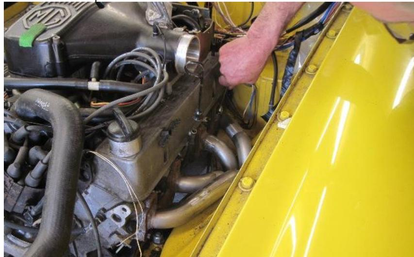
Next job was to see if the exhaust manifolds would fit without having to jack the engine up.
