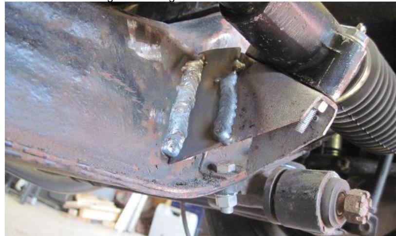
One 1/8" plate welded in for the steering rack mounting.
