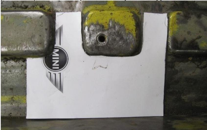
As there are so many joining box sections underneath this area, and the spot welding on them seemed good. I decided against 'invisible' repair and decided to weld the repair panel on top of the holes. Not really best practise, but it would have taken all day to repair this one little bit.
