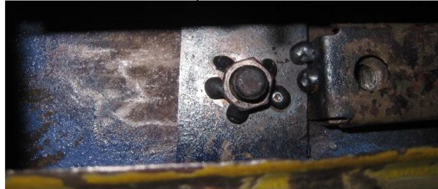
The Kurust turns the rust into something black I have forgotten the name of. All these rust converting products are a help to rusting areas. **If you can get to an area to actually remove rust do so.**
