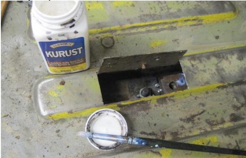
Cleaned up the inside of the box section, as best I could, with a scraper and wire brush. Blew the loose rust and muck out with the air line.
