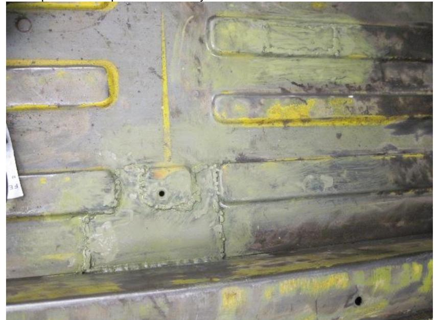
Remember – 25mm of weld will take about a 1-tonne load. So it should be a lot stronger than spot welds.
