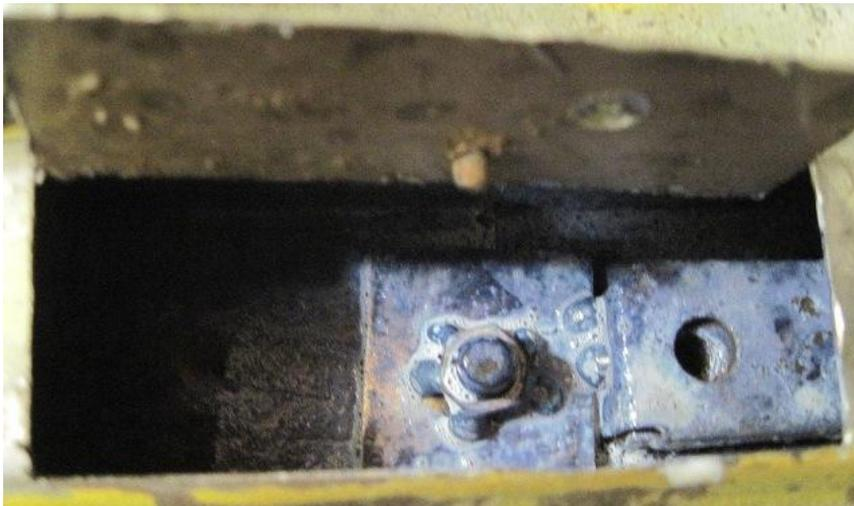
Coated the areas that I could get to with Kurust. This is one of the most widely available rust converters on the market and has rightfully earned itself a good name for clamping down on corrosion. It's easy to apply, being runny, odour free and fast acting. Conversion of the rust starts immediately and is usually complete in around 20 minutes. I have used both Kurust and Jenolite, but there are now products on the market, according to Practical Classics that are more effective and
