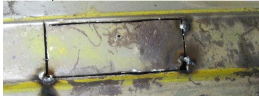
The floor over the chassis rail is tacked back in position. You can see, in the RH bottom corner that I had the MIG welder turned up too high. I really have not done much welding on car body panels for over 25-years. You don't forget how to do it; you just can't do it as well as when you were doing it full time. Anyway, that's my excuse!
