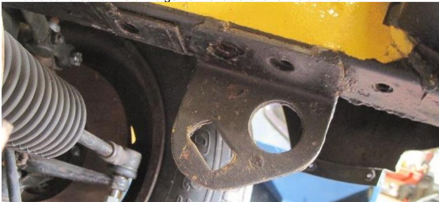
The previous photo is of the towing and tie down eyes on the front chassis rails. I keep banging my head on them when I am working under the front of the car. I have the scars to prove it! They had to go. Out with the angle grinder again.
