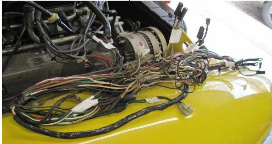
Stripping the loom and labelling the wires started.
