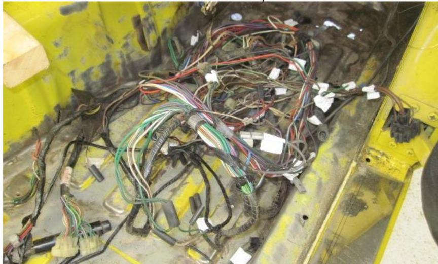
The last photo is of all the engine bay cables stripped back ready to rewire to the new fuse box on the passenger's side.
