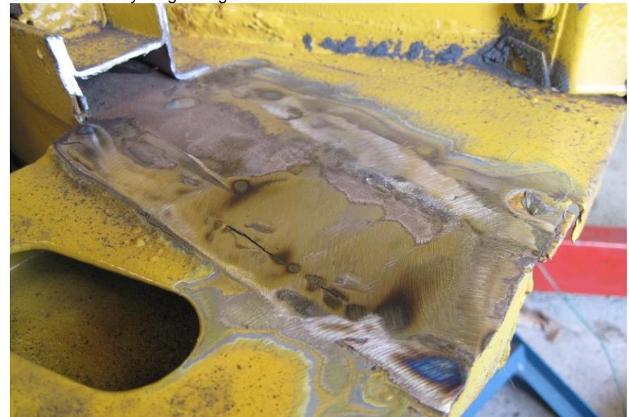
I found under the paint there was rust. The paint will eventually have to be stripped with paint stripper to reveal the rust and grind it out with the mule skinner. Parts that I cannot get to with the mule skinner will have to be treated with a rust treatment, before etch priming, priming and top coating.
