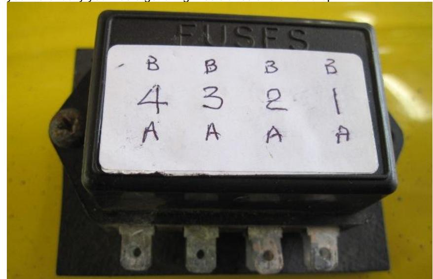
Even the fuse box connections are corroded. The markings are so that I know which wire went of which fuse. Each wire that came off was marked with the code number eg. 4B, 4A, etc.
