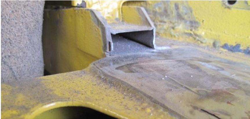
Welds and edges tidied up ready for a plate to be welded over the open box section. Note the corners taken of the top of the box section.
