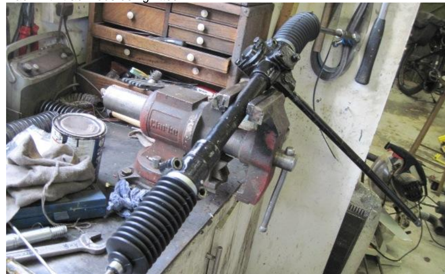
Completed rack overhaul with its new rubber boots fitted ready to fit back on the car. I am sorry if I have left anything out of the rack overhaul. But you can always read the workshop manual before you start. I hope this week to really get stuck in to the MGB and get some more work done on it. It would be nice if I can get the engine running by the end of the month. As usual, comments, questions, suggestions and abuse to: mikemacartney@btconnect.com
