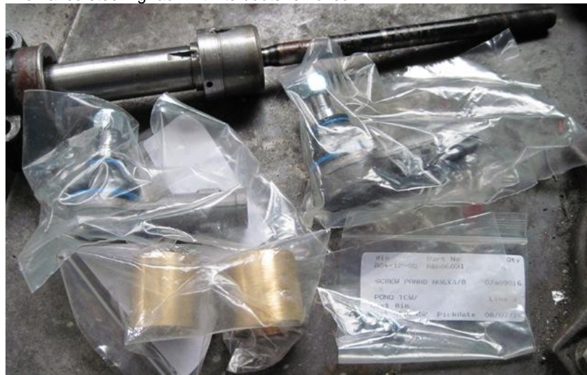
The naked steering rack with its boots removed.
