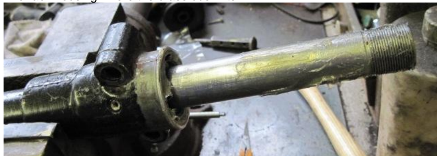
Rack greased up and checked for sliding smoothly.
