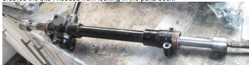
The naked steering rack with its boots removed.
