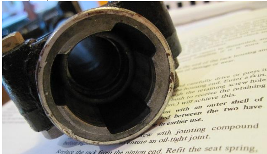
The rack housing where the brass bush fits.
