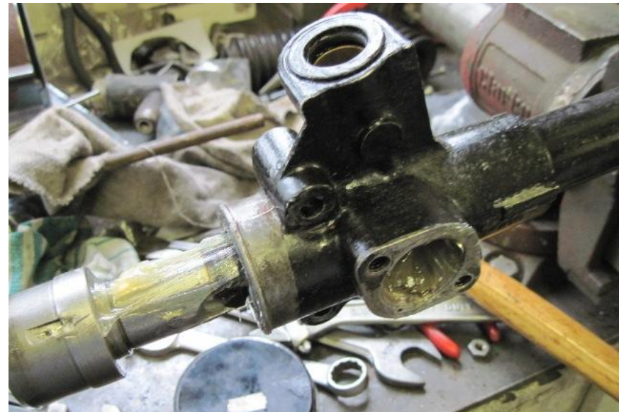
Rack with track rods being fitted.
