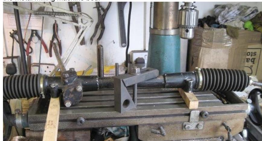
Then I found the largest drill that would go through the smallest part of the elongated hole in the steering rack casting and centred the drill in the oval. I then drilled through with progressively larger drills until I had made the hole in the casting round. The top hole in the photo below is the hole I have drilled and the lower one has yet to be drilled. I was careful to only take enough metal out to make the hole round.
