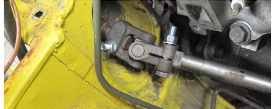
I have new 5/16" UNF fitted bolts and nuts in temporarily to hold the rack in position. These bolts I will machine down to the correct length in the lathe and when it comes to fitting the steering UJ for the last time I shall use Nyloc nuts.
