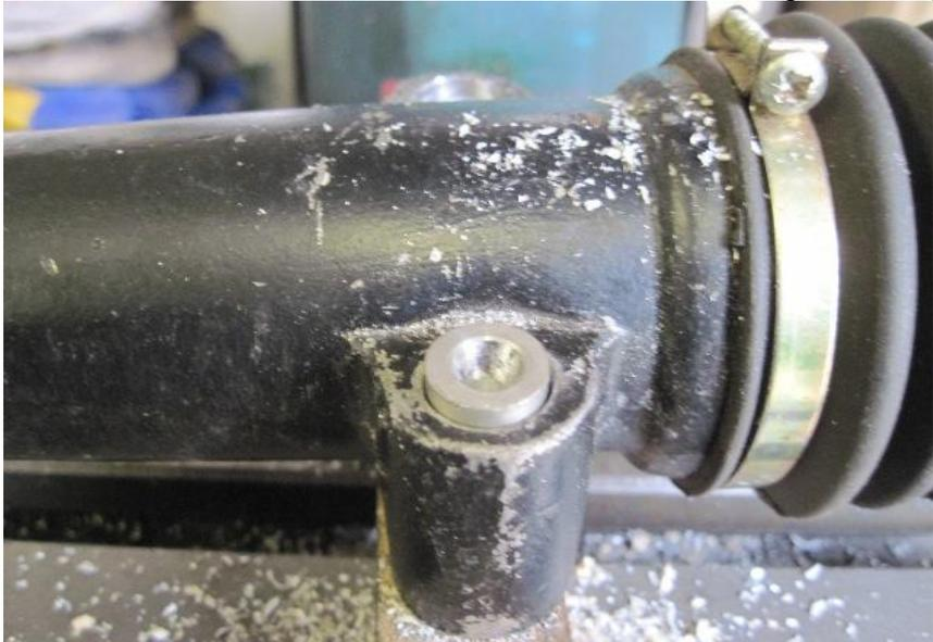
I checked the fit of the inserts and then machined them down in the lathe to the correct height. Although they were a push fit into the steering rack I did not want them to move or rotate when I drill the holes through the inserts, so I pushed them in coated with Araldite (not the rapid type Araldite). The steering rack is now in our downstairs bathroom waiting overnight for the Araldite to set.
