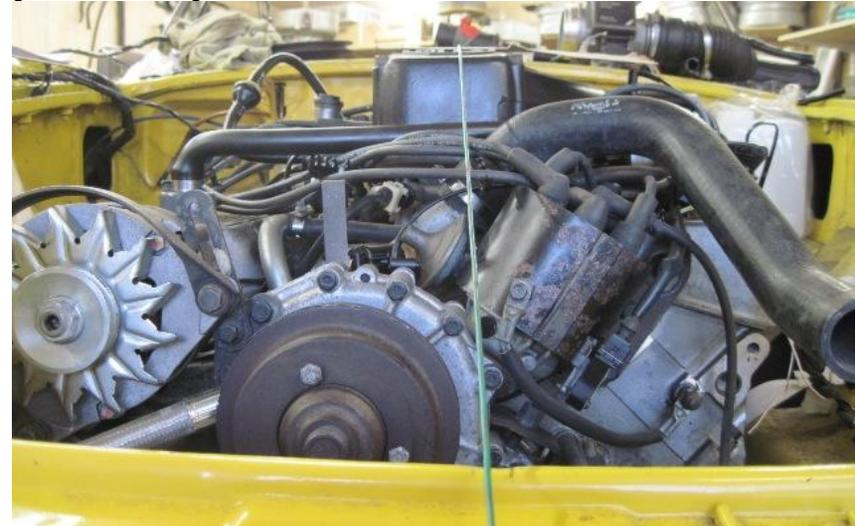
I stretched a length of cable down the centre line of the engine bay to check the position of the engine. It needs to move to the LH side by about a 1/4".
