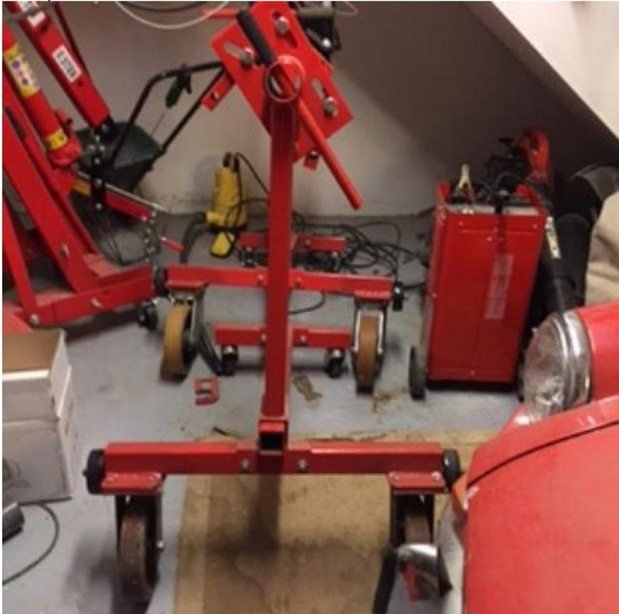
Roel Hellemans spit for his MGB bodyshell with two engine stands with 6" casters attached. This maybe the way to go for me if I can't find a suitable cheap spit.
