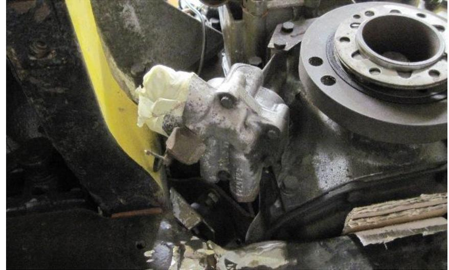
There is just not enough room to fit the steering rack in without raising the front of the engine. I have spent enough time trying to achieve it, but now is the time to give in. I shall decide later whether I lower the injection system by machining the castings or plump for a power bulge. Now I shall just concentrate on getting the engine, gearbox and steering rack fitted in their correct places.
