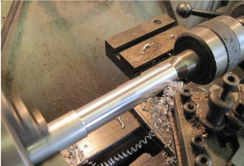
When I had machined the inserts to the correct diameter, I sawed the machined bar in two and faced one end of each and used a centre drill to as a start for the correct size drill for when it came to machine the holes in the steering rack casting.
