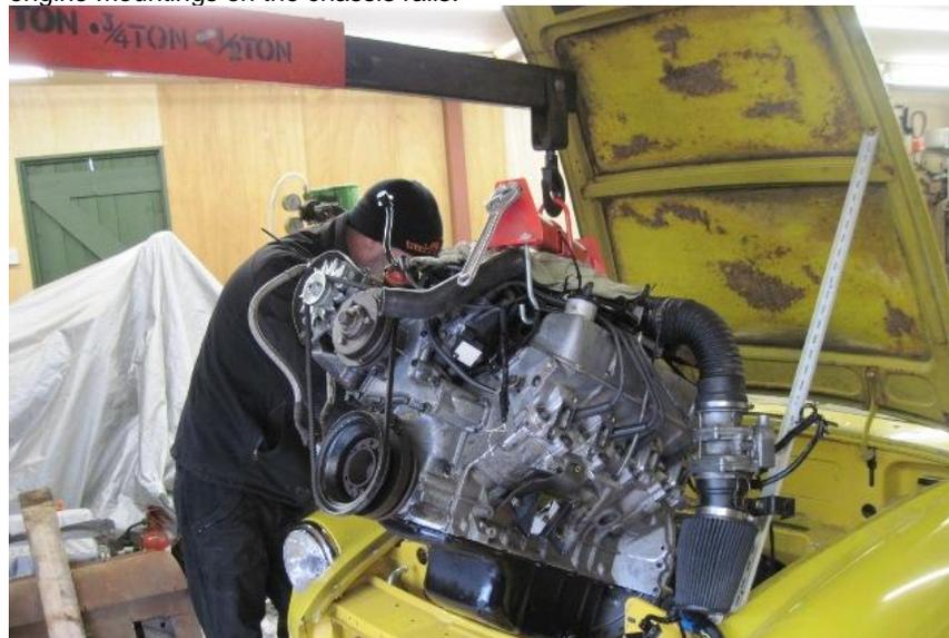
I had bolted the new metal mountings to the rubber engine mountings, so I could either tack weld them in place, if there was room, or mark the position where they were to fit then remove the engine and gearbox again to finally weld them in position.
