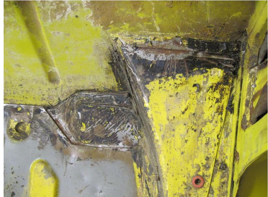
Here I have cut away the thick black seam sealer that BL used. You can see that rust has developed in the seam and needs to be treated before new, more modern seam sealer is applied.
