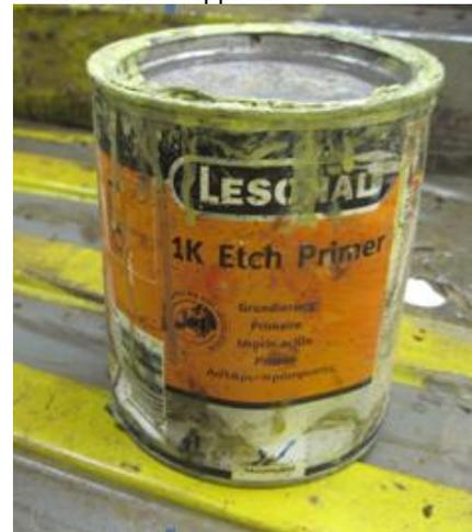
**Any bare metal needs to be treated with a thin coat of acid etch primer** as soon as possible after grinding, sanding or paint removal. This will stop any rust developing before you have a chance to paint with primer and topcoat. A 1-litre tin will last for a long time. I only used half a litre on the MGBGTV8 restoration.
