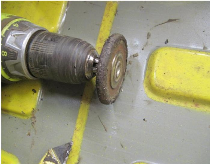
Going back to bodywork, this tool is called a **Muleskinner** and is ideal for removing rust and paint. It is a wire brush encapsulated in resin. I used only one on the complete restoration of Dugald's MGBGTV8.
