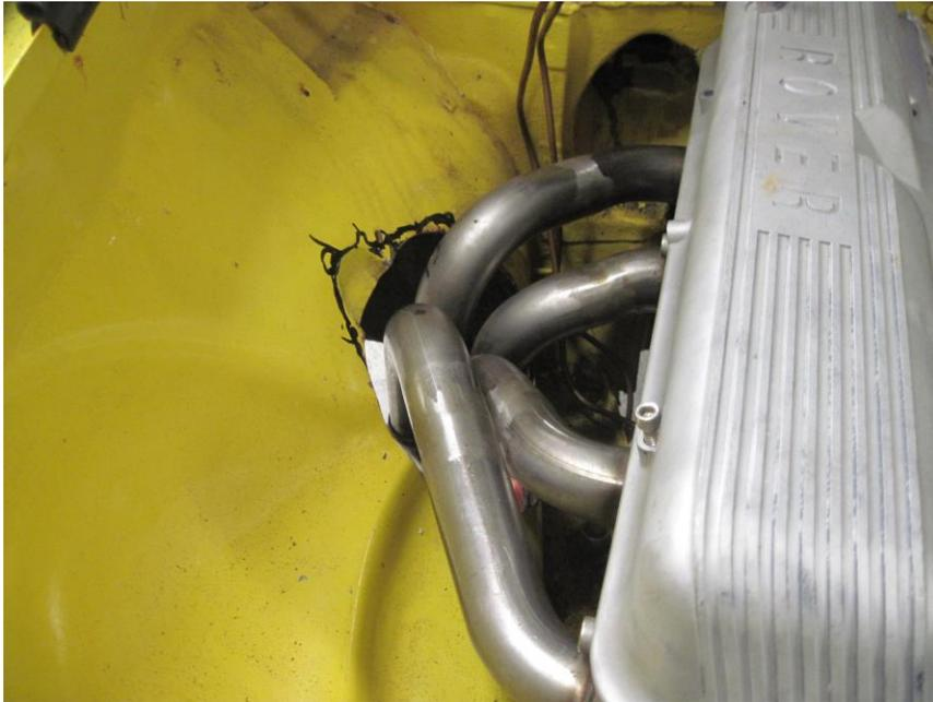
Eventually, we managed to **fit the right-hand the manifold in place**. The same problem with the weld on the manifold collector touching the inner wing happened on this side as well. The black marks on the inner wing are where the hole in the inner wing needs opening up so that the manifolds can be removed without jacking up the engine.
