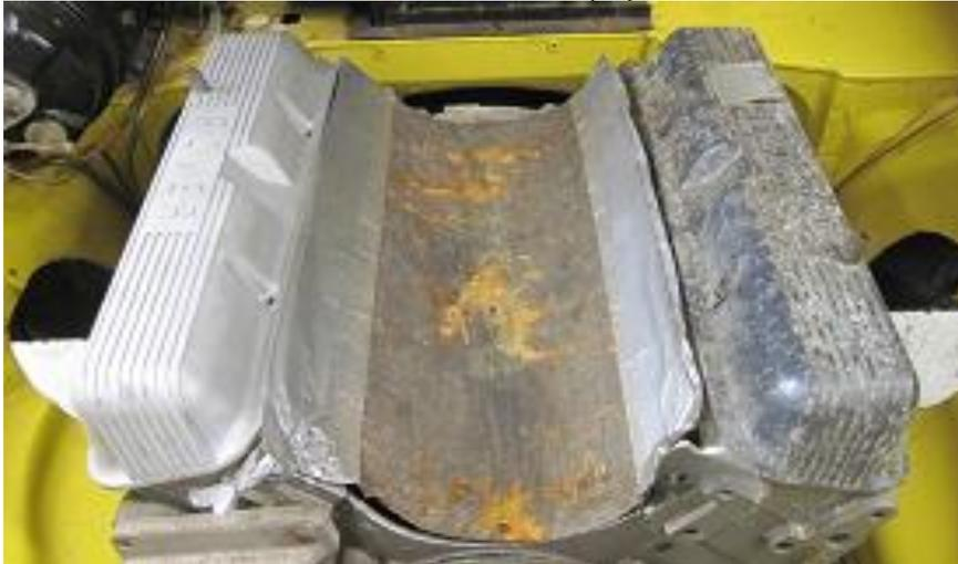
What a bead blaster can do. The rocker cover was originally like the one on the right of the photo. I wish I had had a bead blaster when I restored Dugald's MGBGT V8 it would have saved me a lot of time.
