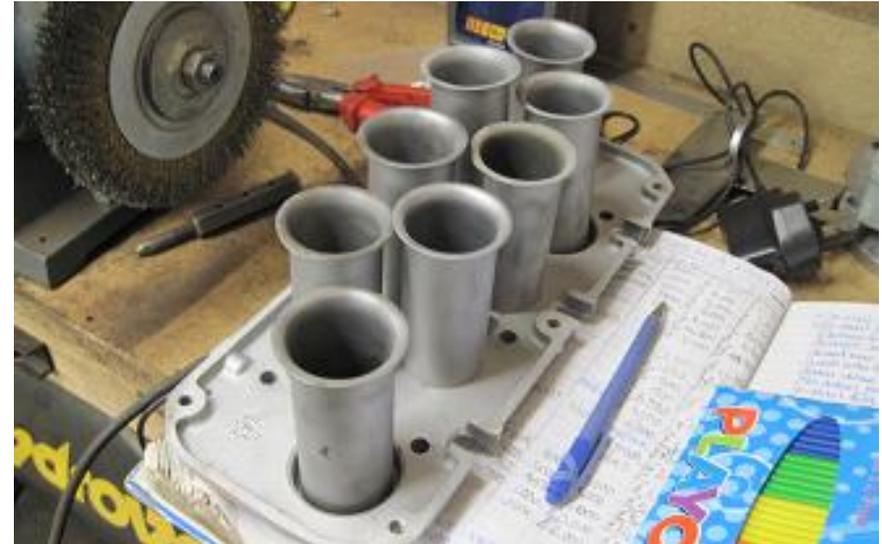
The EFi trumpets bead blasted. The mounting plate is scrap due to the last owner machining (or had machined) too much metal off both the bottom and the top of the casting. Underneath is my book that I make copious notes in about what I need to buy, where things fit, etc. etc.
