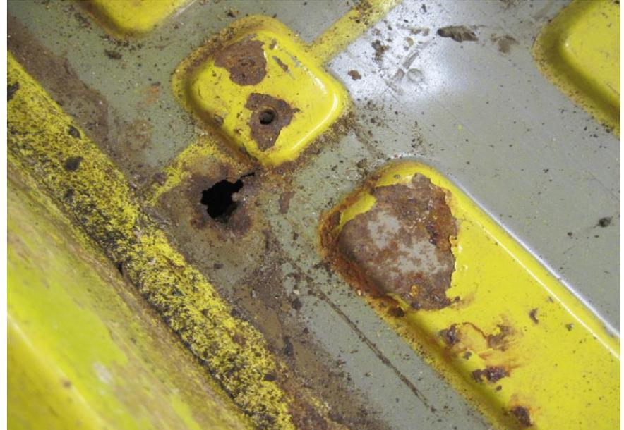
Rust holes covered up by perfectly good tar. More welding to do later! The tar comes off very easily with a hammer and sharp chisel.
