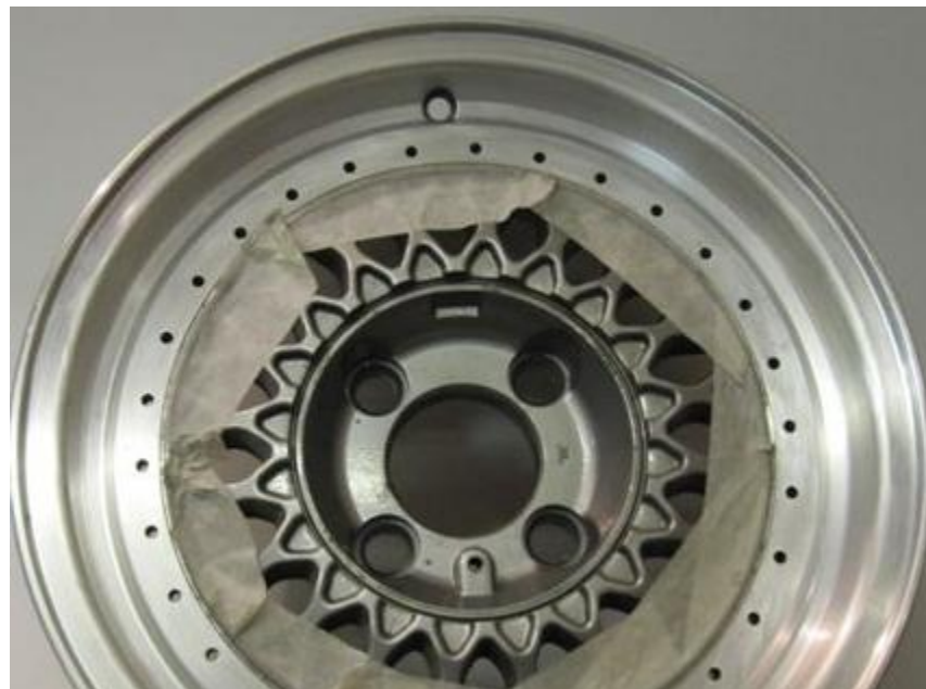
Masking tape protecting centre section which is not to be stripped
