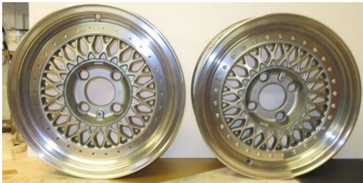
Left: stripped wheel without studs. Right: fitted with socket button head bolts.
