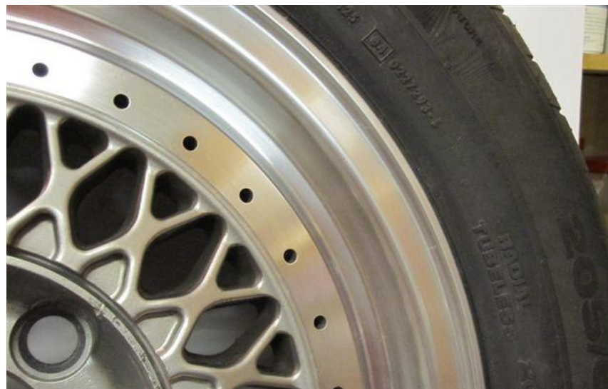
Studs removed and stripped
