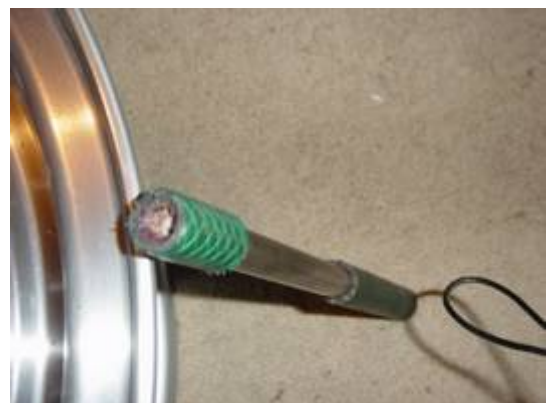
Tool made with a piece of water hose to drive the false studs back in. Cut leather wad in the end to cushion stud head. Green garden hose to stop stud slipping off driving pin. (Photos: David Sutcliffe)
