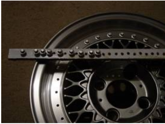
Close up of wheel showing tool to hold false studs.
