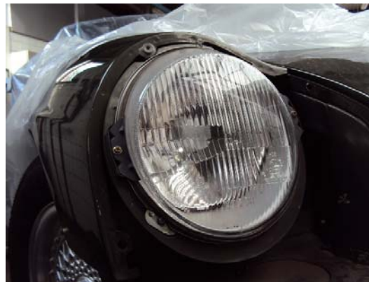
LHD lens (above) of the right side headlight fixed to the car after conversion which shows the difference between RHD lens (below).
