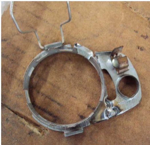
Bulb holder welded back together again, displaced by a few millimetres. Top and bottom of the side light bulb holder has been shortened by some millimetres
