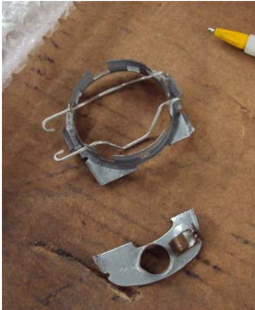
Bulb holder cut into two pieces
