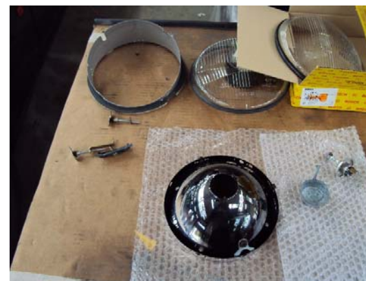
Headlight completely dismantled
