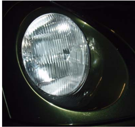
LHD lens (above) of the right side headlight fixed to the car after conversion which shows the difference between RHD lens (below).
