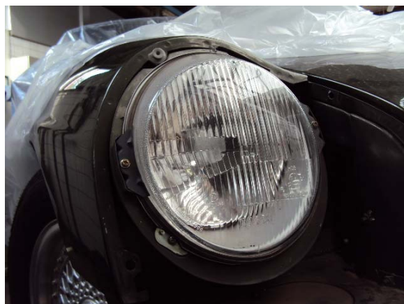
RHD lens of the right side headlight fixed to the car before conversion.
