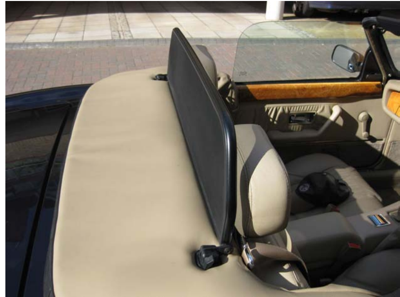
Completed tall windstop from the offside.
