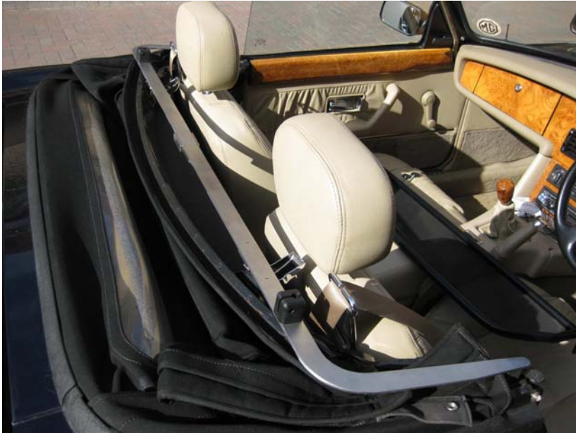
New rail in stainless steel replaces the standard tubular tonneau rail.
