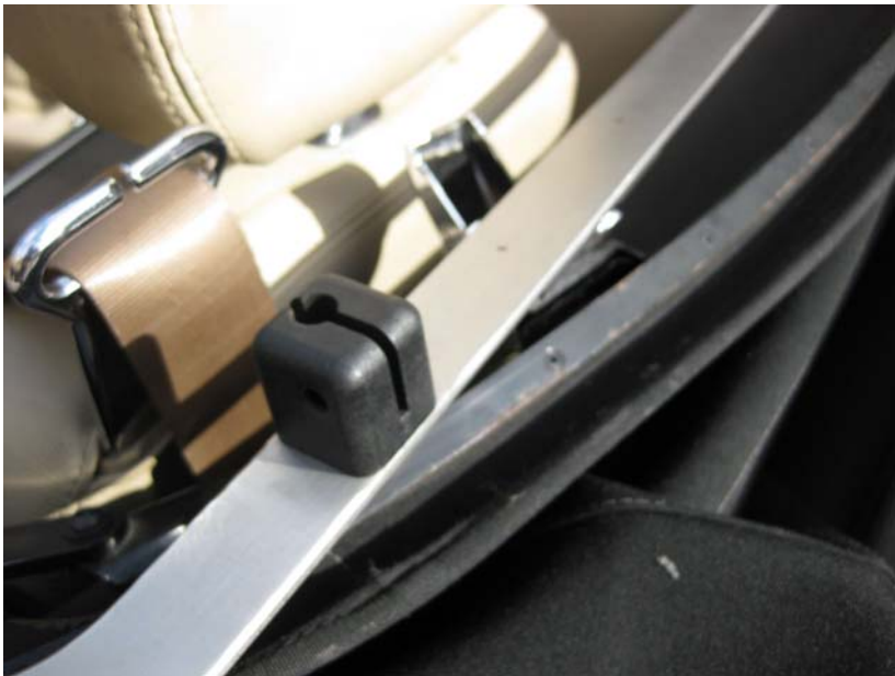
Windstop fixing block supplied with the windstop kit on the new rail.
