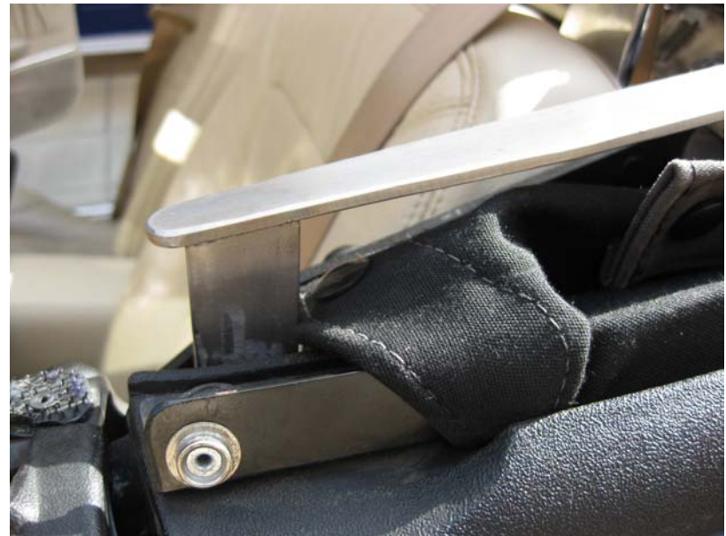
Nearside lug on the new rail fits into the tonneau rail socket.
