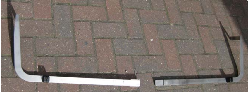
New rail splits for convenient stowage.
