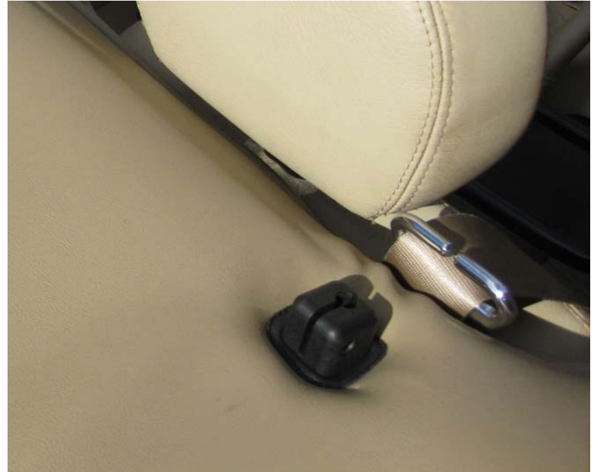
With the windstop removed the fixing block sits neatly in the tonneau. Angus had these holes made by a local trimming company who was a tonneau specialist as he wanted the result to look a professional job.
