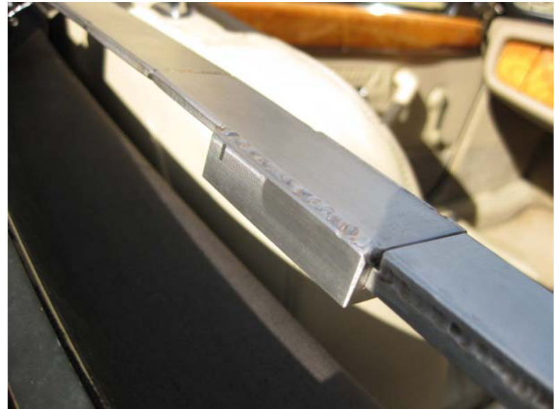
Cartridge and tongue fixings so the new rail can be split for stowage.
