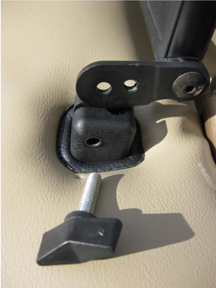
Removing the windstop involves unscrewing the wing nut securing the windstop to the fixing blocks on the new tonneau rail
