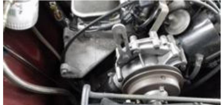
When you get the alternator out it should look like this . . . . . and the location it came from looks like this. The cradle bolts to the RH cylinder head and supports the alternator by two bolts.
