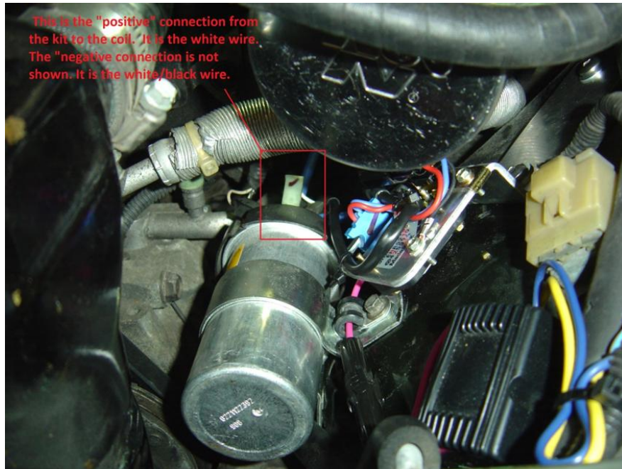
This is the positive connection from the kit to the coil. It's the white wire. The "negative" connection is not shown. It is the white/black wire.
