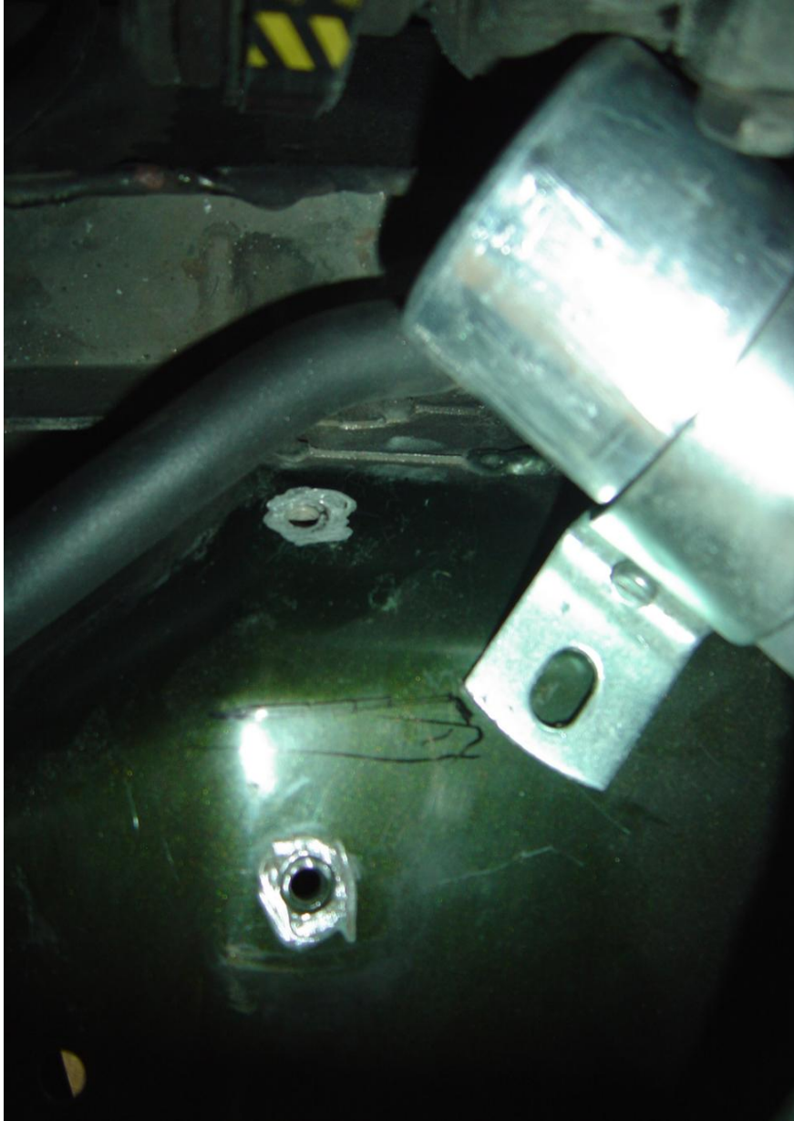
The location selected to mount the kit. It is the two coil mounting holes with the paint removed to provide a good ground connection.
