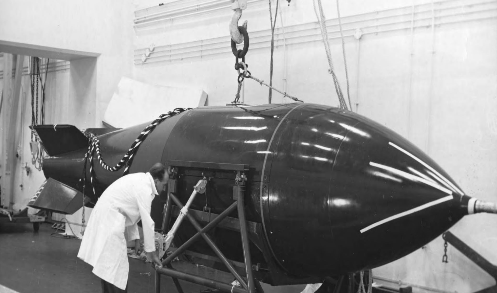
This is Britain's first production atomic bomb. Code named " Blue Danube ", it had the same explosive power as those dropped on Japan – about 16,000 tonnes of conventional high explosive. The RAF's three V-Bombers – the Vickers Valiant, the Handley Page Victor & the Avro Vulcan – were each designed to carry this huge device to Russia, in response to a Soviet nuclear attack – the strategy of deterrence was born.
