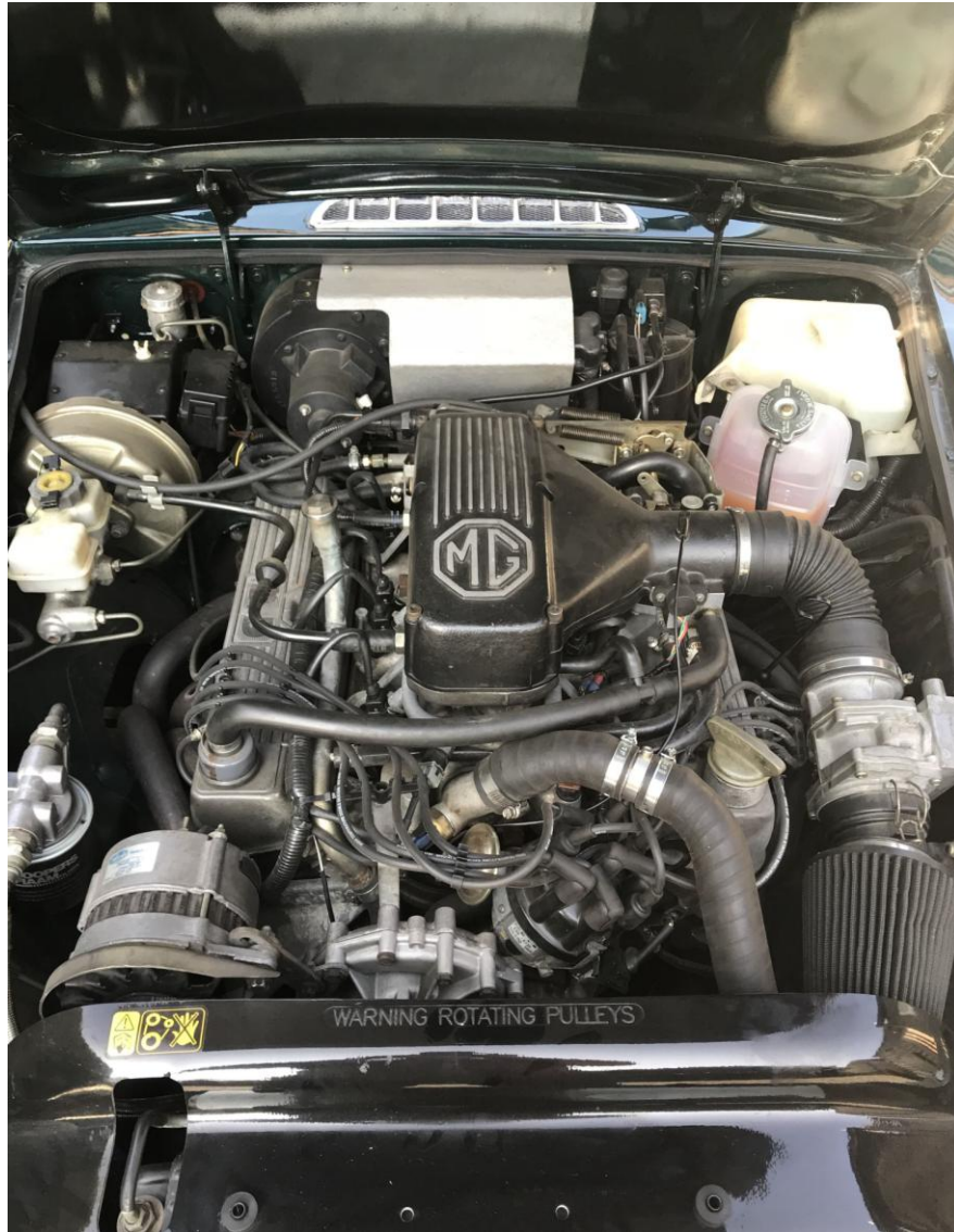
Engine bay with new carbon fibre radiator cowl.
