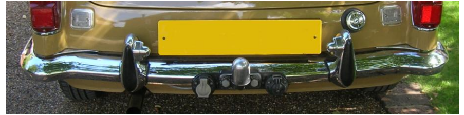
Witter towbar car fitted to an original MGBGTV8 chrome rear bumper with twin electrical outlets
