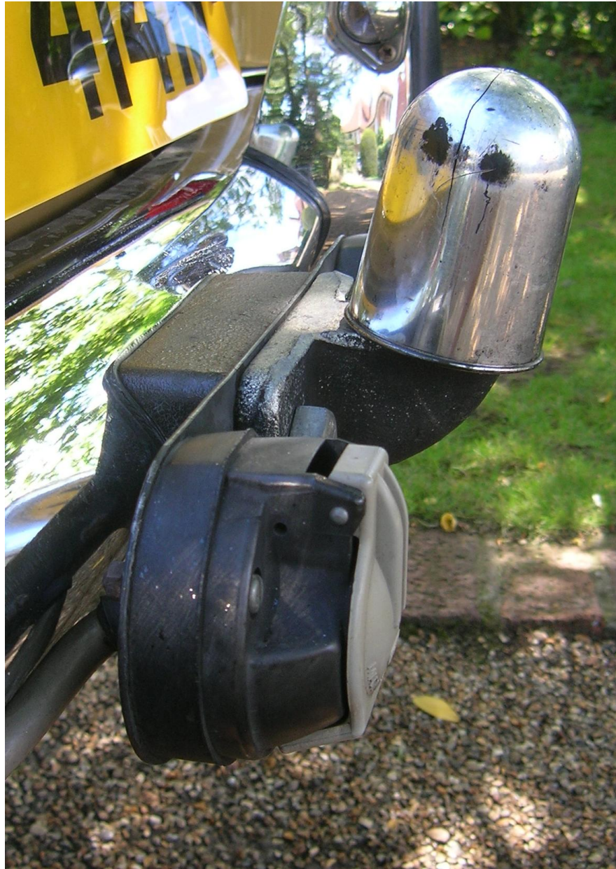
Witter towbar car fitted to an original MGBGTV8 chrome rear bumper with twin electrical outlets for vehicle lighting and power supplies.
